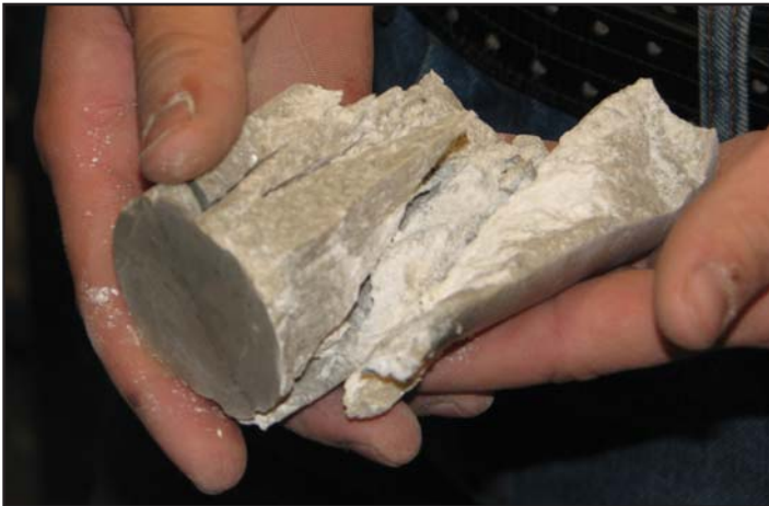
Above: Phil Riehl, Geotechnology Inc., prepares a sample of limestone for an unconfined compression test. In this test, geologists determine how much pressure the rock can take without shattering. Left, Riehl examines the remains of the limestone after the test.
