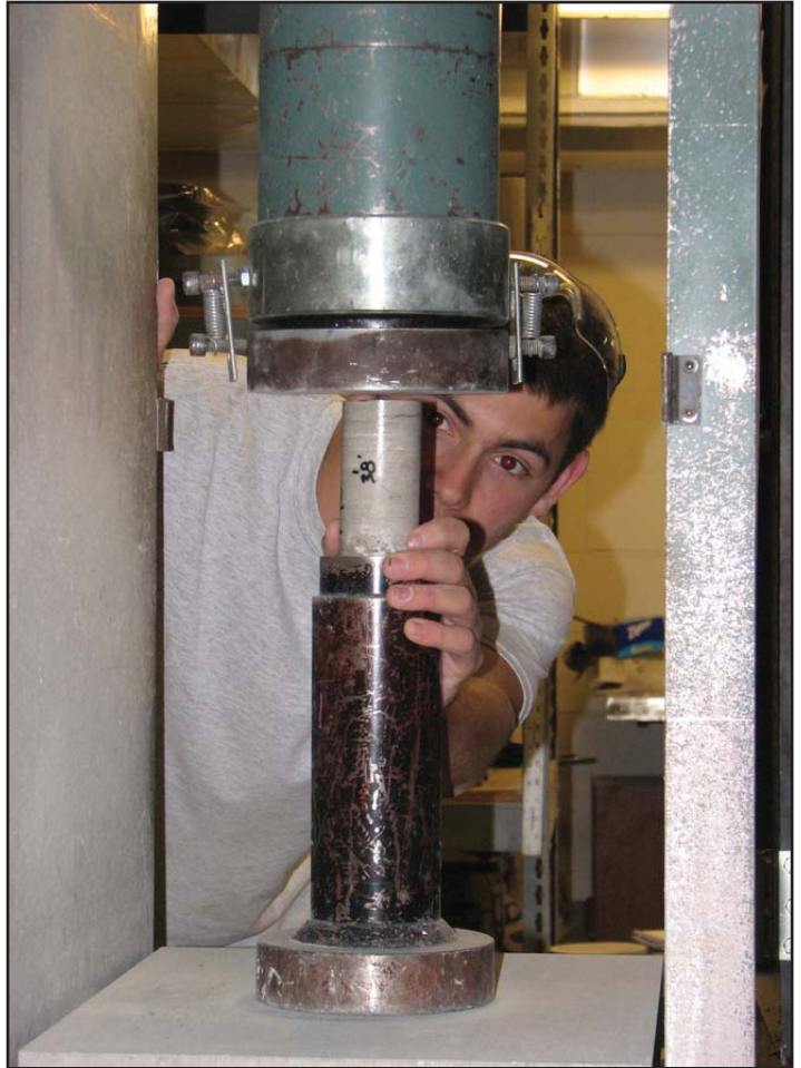
Above: Phil Riehl, Geotechnology Inc., prepares a sample of limestone for an unconfined compression test. In this test, geologists determine how much pressure the rock can take without shattering. Left, Riehl examines the remains of the limestone after the test.
